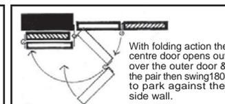
With folding action the centre door opens out over the outer door & the pair then swing 180° to park against the side wall.
